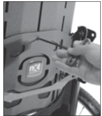
Fig. 6: Loosen 3 cap screws to adjust back height
