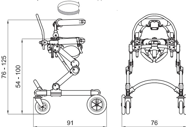
**GRILLO FRONT-DRIVE gait trainer size *ThreeFour* WEIGHT 19,5 kg MAX. LOAD kg 90**
