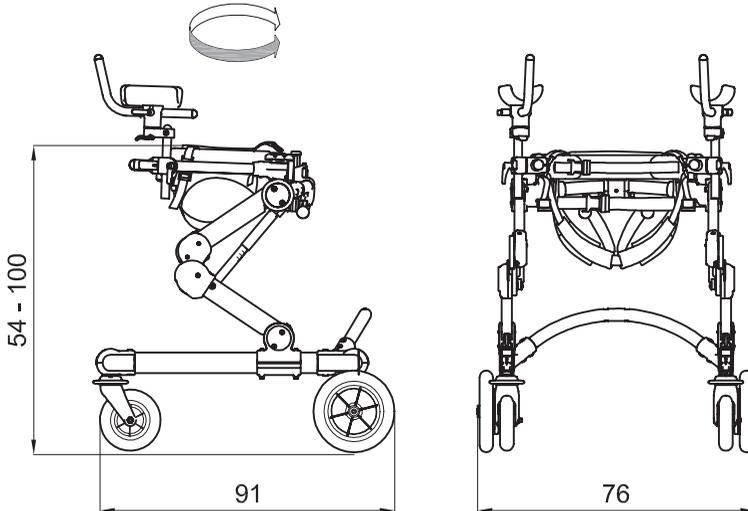
**GRILLO POSTERIOR** gait trainer **size ThreeFour** WEIGHT 17,7kg MAX LOAD. kg 90
